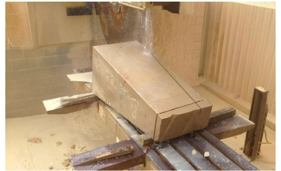
Sandstone is quarried by drilling or sawing. It can then be saw- or water-jet-cut to precise dimensions
