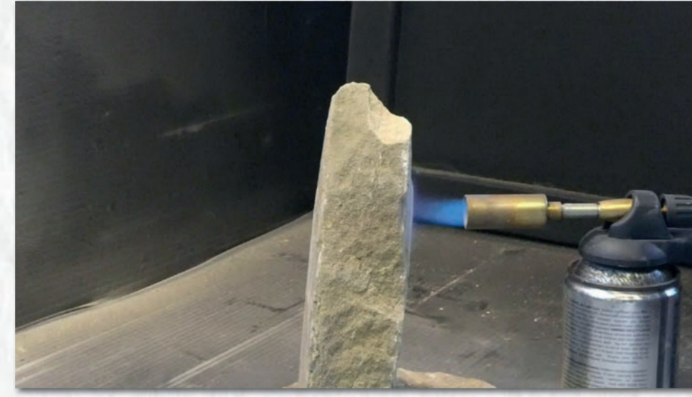
Non-flammable with a high-degree of thermal capacity. Useful for smoothing day-night temperature swings
