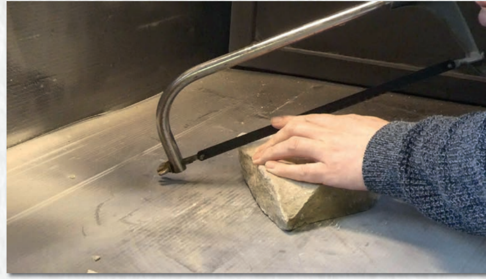
Inelastic. Will chip if struck at a vulnerable point, but will not fracture or shatter
