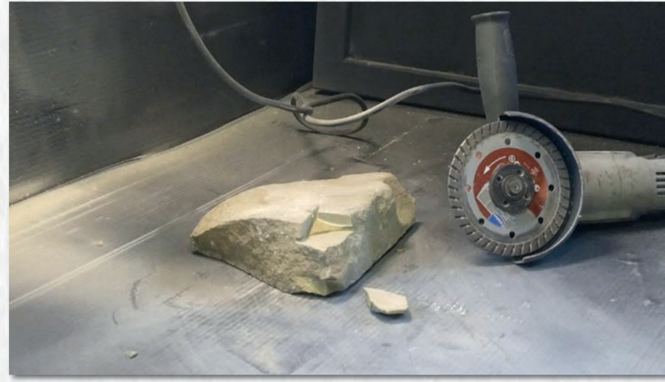
Inelastic. Will chip if struck at a vulnerable point, but will not fracture or shatter
