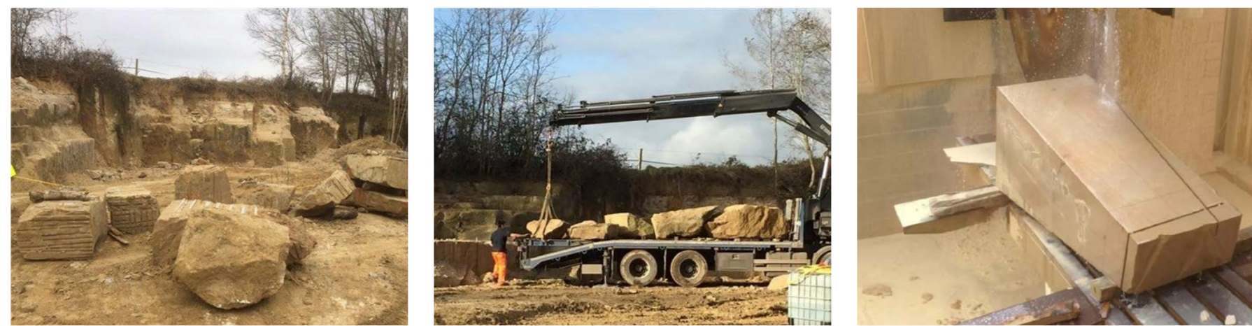
Sandstone is quarried by drilling or sawing. It can then be saw- or water-jet-cut to precise dimensions
