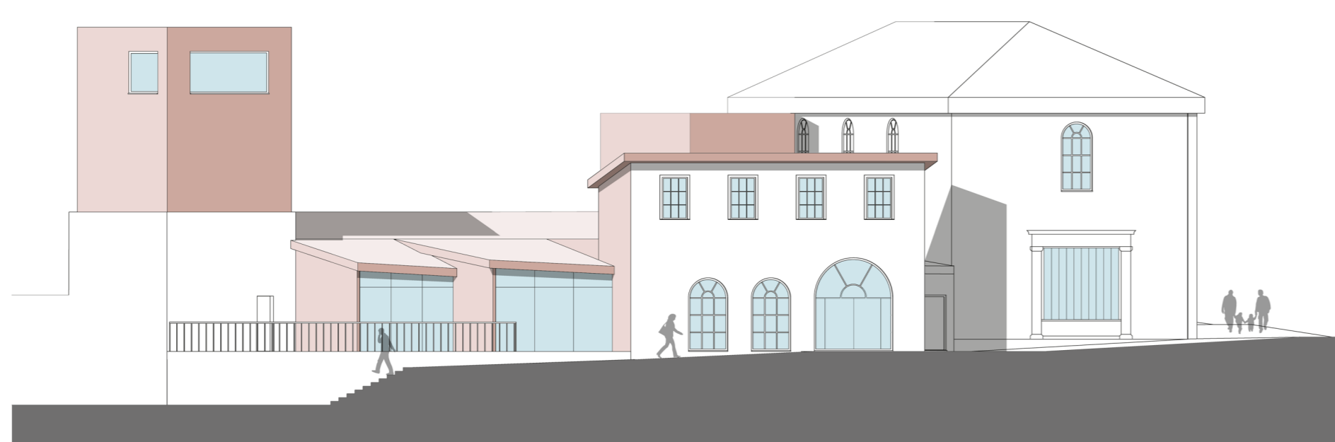
E2 - Facing south, the development resembles the original triptych, with the steel tower to the east, reclaimed brick frontage in the center, and Crystal House to the west. (1:200 @ A1)
